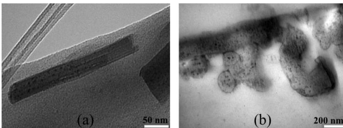
**Figure 2.** (a) Perpendicular view TEM image of dispersed nanofibers. (b) TEM image of a nanofiber cross-section embedded in Poly/Bed 812 and positively stained. Filled core nanofibers with small isolated dark contrast regions throughout are observed in both images.
