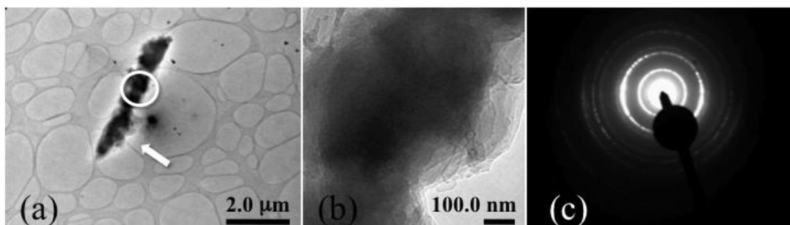
**Figure 3.** (a) Plan-view TEM image of nanofiber with large dark regions. (b) Close-up of region identified by the arrow shows an irregular electron transparent surface and dark non-electron transparent regions in the interior (c) The SAED diffraction pattern of a dark region indicates a polycrystalline material.
